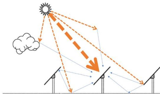
Historical measurement practices employ fixed-position or slowly moving sun tracking sensors which are incapable of accurately or directly determining the tilt angle of maximum irradiance. In contrast, the MPIS™ quickly samples plane-of-array solar Irradiance (POAI) at multiple small angular increments about a fixed rotational axis.
